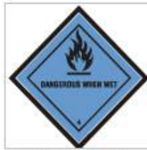
Dangerous when wet
